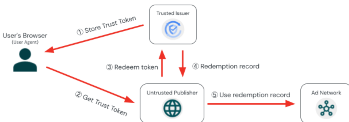
Figure 5: Using a Trust Issuer to validate the authenticity of a user and retrieve a Redemption Token as proof of the user's validity.
